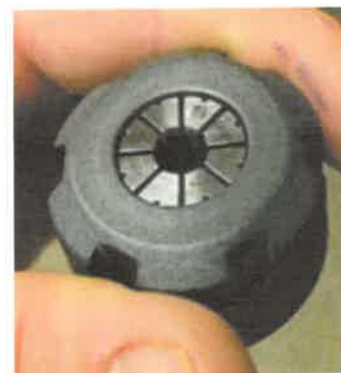
Spindles: snap collet into nut, then flip it over to ensure it is snapped in securely
