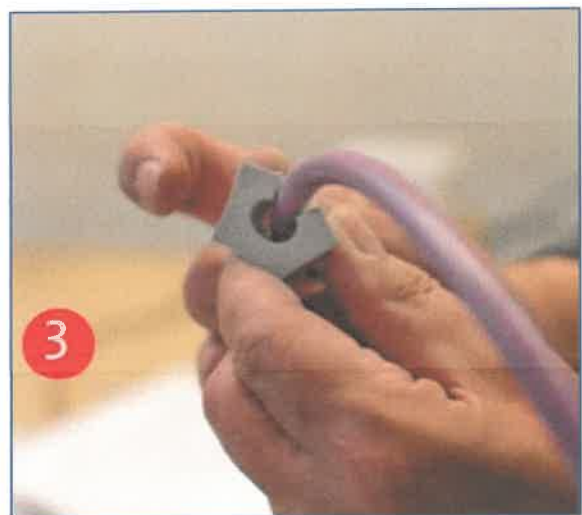
Equip the corresponding KT grommet with the cable.
